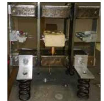
3. New SMA-based ATMD layout
