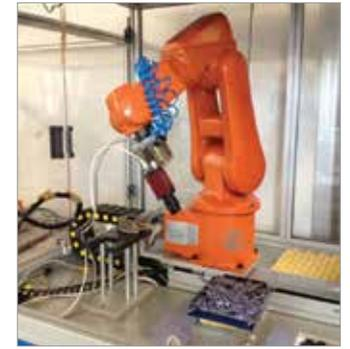
**3. Robot bin-picking application using stereoscopy**
